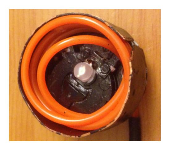
Put the cap on, turn on the LED light, plug in your EL wire, and place into the hole in your ISAC.
