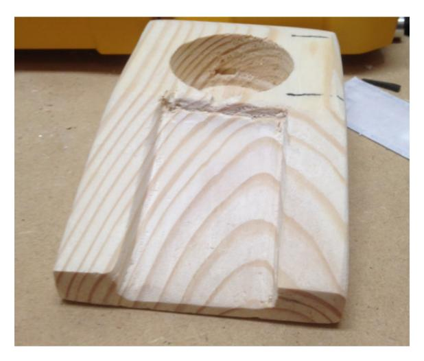
Take wood filler and fill in anywhere you need to - I had to fill in the edge of the circle because the drill shredded the edge at one point. After that dries, sand, sand, sand until you are sick of sanding and then sand some more. The smoother the surface the better. You can also sand in details, if desired.
