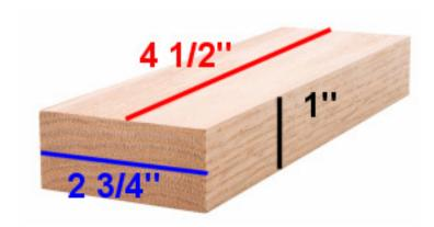
Once you have your board, you need to figure out where you are going to put the light. I picked a side to have the light and marked two lines, one at 7/8" and the other at 2 3/8" (roughly, I am horrible at reading rulers).
