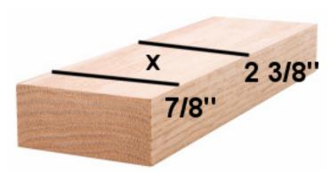
Drill a pilot hole all the way through the wood where x marks the spot. Take your 1 1/8" spade bit and drill a hole. Go low and very slow (high torque low speed) with the spade bit as it will catch the wood and, if you forget to set your drill to stop spinning when it gets stuck, you can give yourself a black eye (true story).
