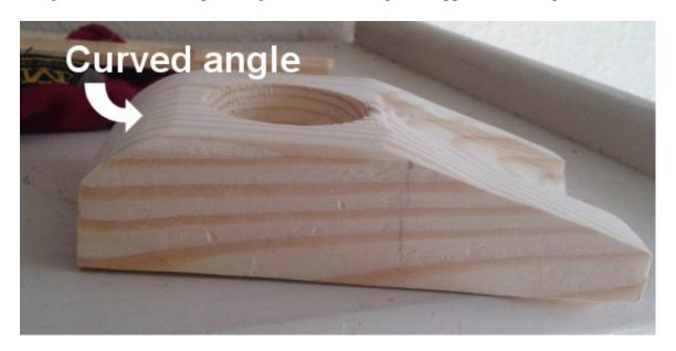
From the 2 3/8" line to the edge, sand a angled line. If you need to, you can adjust where the angle starts (if it's too close to the edge of the hole, you definitely want to move it away some). My angle is roughly 30 degrees but I went with more of a 'does it look right' vibe than an actual measurement.
