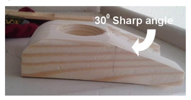
To cut the groove in the wood, first draw a line in the center of the wood to the edge. Measure 1 1/4' on either side and draw a line there as well.
